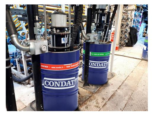
Diagram 2.4: Main Bearing and Labyrinth Grease on a TBM
